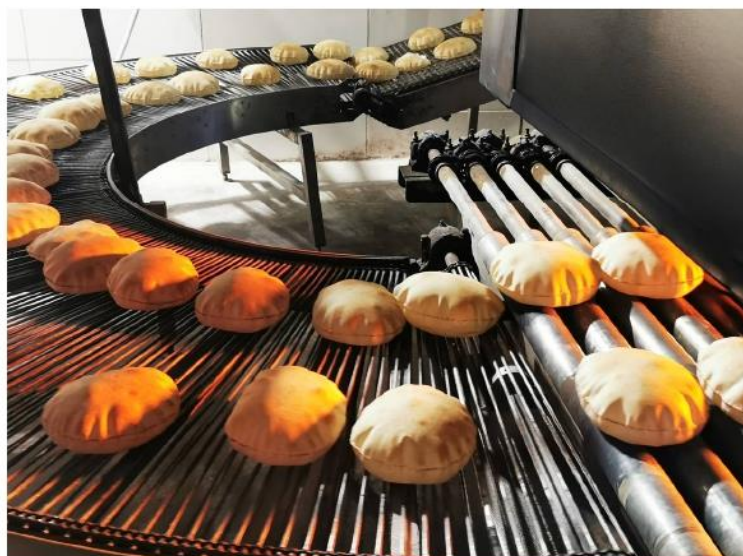
Figure 3. Jordan Kmaj in an automatic baking line. The inflation of bread due to the thermal expansion of the gases is clearly visible.
