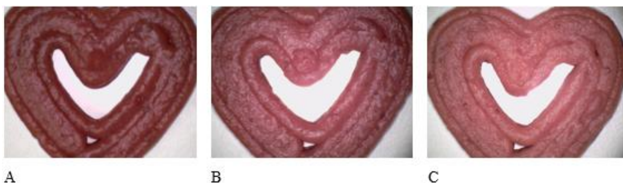
Figure 1. Microscopic pictures (500×) of 3DP samples: Influence of added starch, 10% (A); 15% (B); 20% (C), on the lightness ( L^* ).
